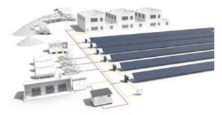
John Cockerill is supporting Chad in the gradual deployment of mini-grids, i. e. relatively small, local, green electricity production units (between 10 kW and 10 MW) that are isolated from other power grids.
