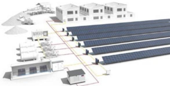
John Cockerill is supporting Chad in the gradual deployment of mini-grids, i. e. relatively small, local, green electricity production units (between 10 kW and 10 MW) that are isolated from other power grids.
