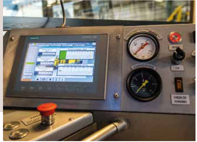
Touch panel (speed, tractive effort, consumption, motor settings, ...)
