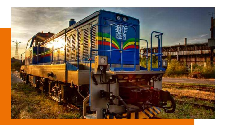
With its 1200 HP and high efficiency AC/AC transmission, this locomotive is adapted for every needs. Ideal to haul a passenger train on long distances, the DE1200 can also be used in multiple units to haul up to 10.000T freight trains. This makes this model the must have in your fleet.
