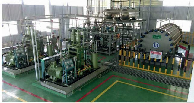
Production and compression installation for 500Nm<sup>3</sup>/hour (electrolyser, separators, purifier, compressors)
