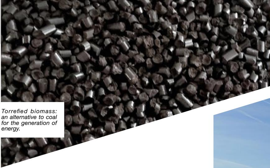
*Torrefied biomass: an alternative to coal for the generation of energy.*
