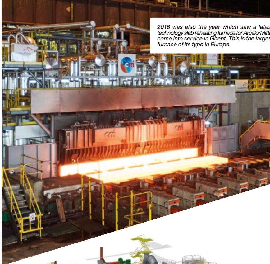
2016 was also the year which saw a latest technology slab reheating furnace for ArcelorMittal come into service in Ghent. This is the largest furnace of its type in Europe.
