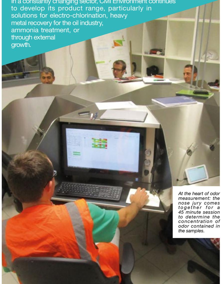
At the heart of odor measurement: the nose jury comes together for a 45 minute session to determine the concentration of odor contained in the samples.
